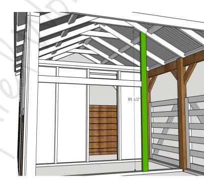
Step 4: Add fence pickets with screws straight through and into the divider frame leaving a 6" gap between boards Stagger them opposite on the other side there is no gap!
