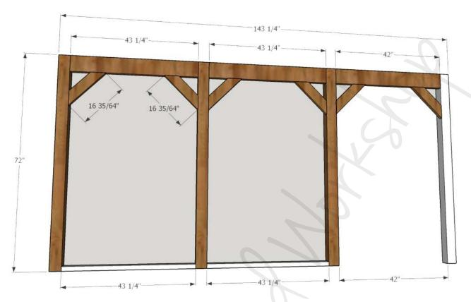
Step 5: Attach the front of the goat house to the other walls. Screw through the 2x4s of the side walls into the 4x4s of the front frame. The last post will be standing out there alone for a few steps!
