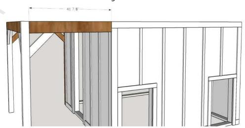
Step 13: Add the 2x6 @ 93 7/8" in between the side posts. Add angled braces here as well.
