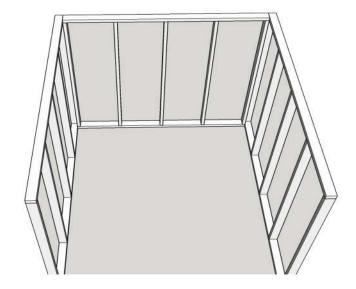
Step 4: Build the front of the goat barn. Use pocket holes or 5"L brackets to attach 2x6s to 4x4s. Screw screws straight through the angled 2x4 boards into the 4x4s. The bottom 2x4s are attached using pocket holes drilled at 1 1/2" depth and 2 1/2" screws on the bottom of the 2x4s.
