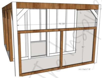
Once the frame is built, attach the frame to the 4x4s with 3 1/2" screws directly through the 2x3s and into the 4x4s.
