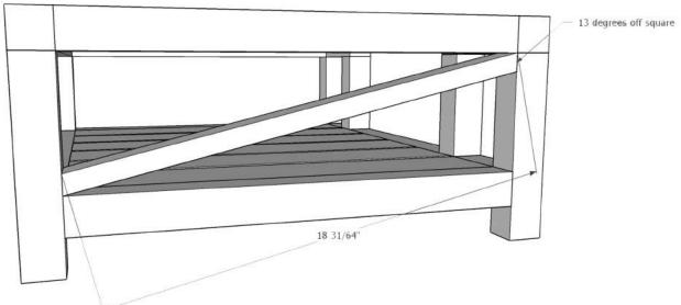
Step 6: Attach X pieces on the sides. See blog post for help on attaching the pieces.
