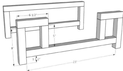
Step 3: Attach the front panel to the back panel with 2x2s @ 18". Pocket holes the same as step 1.
