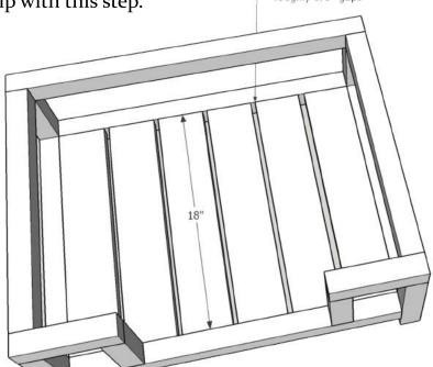
Step 5: Using ample wood glue and a brad nailer attach solid X piece on the sides.
