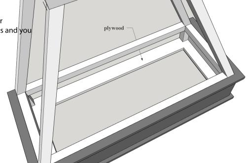
Step 11: Start adding the 1/4" plywood to cover the entire frame. Just brad nail into place. 12 53/64 <del>-17 29/64"</del> 39 29/64" 17 1/2" 12 53/64"
