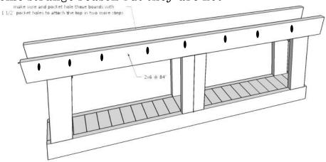
Step 9: Attach 2x6s @ 8 1/8" using countersunk 2 1/2" screws and glue!
