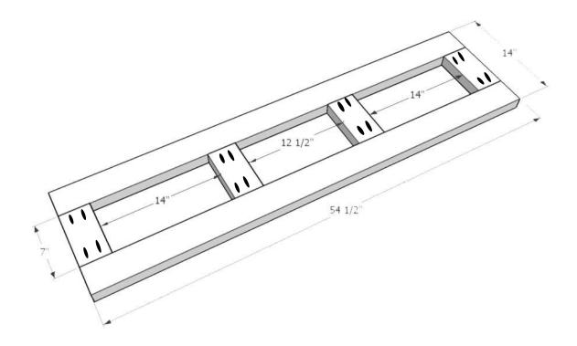
Step 3: Connect the top to the base using 2 1/2" pocket hole screws and glue of course! Make sure to leave a 1/2" overhang!
