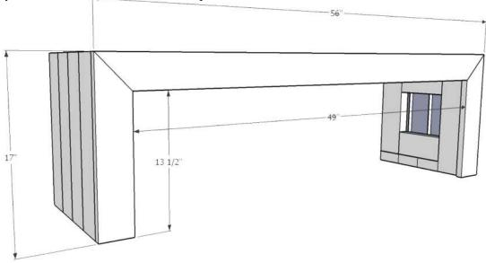
Fill in the underside of the bench with the 1x4s cut at 14 3/4"
