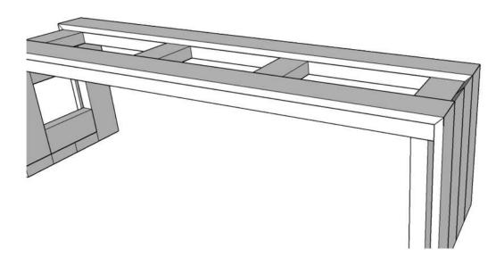
Attach the front and back face frame boards. Using the 1x4s @ 17" mitered at 45 degrees off square on one end and the 1x4s cut to your desired length for the sides and mitered to 45 degrees off square on one end as well! If you would like this to be one solid piece it will be mitered on two ends!
