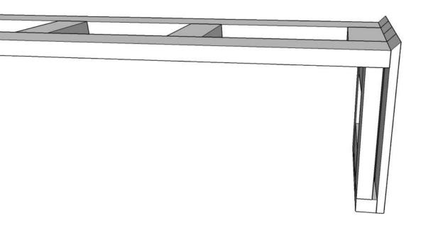
Attach top boards that are cut at any length you choose but beveled on one end...unless you want it to be one solid board across...it will be beveled on both ends! Continue until you have covered the top and sides!
