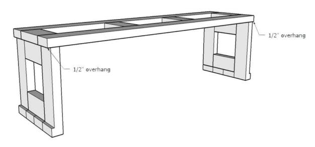
Step 4: Start attaching the outside leg boards that are 1x4 @ 17" with one beveled edge!
